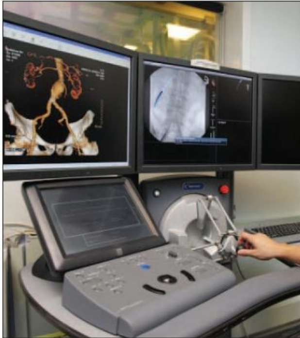
Figure 1. The Sensei robotic system (Hansen Medical, Mountain View, CA) workstation is shown outside the angiography suite during cannulation of the short contralateral limb of an infrarenal Endurant stent graft (Medtronic, Inc., Minneapolis, MN).
